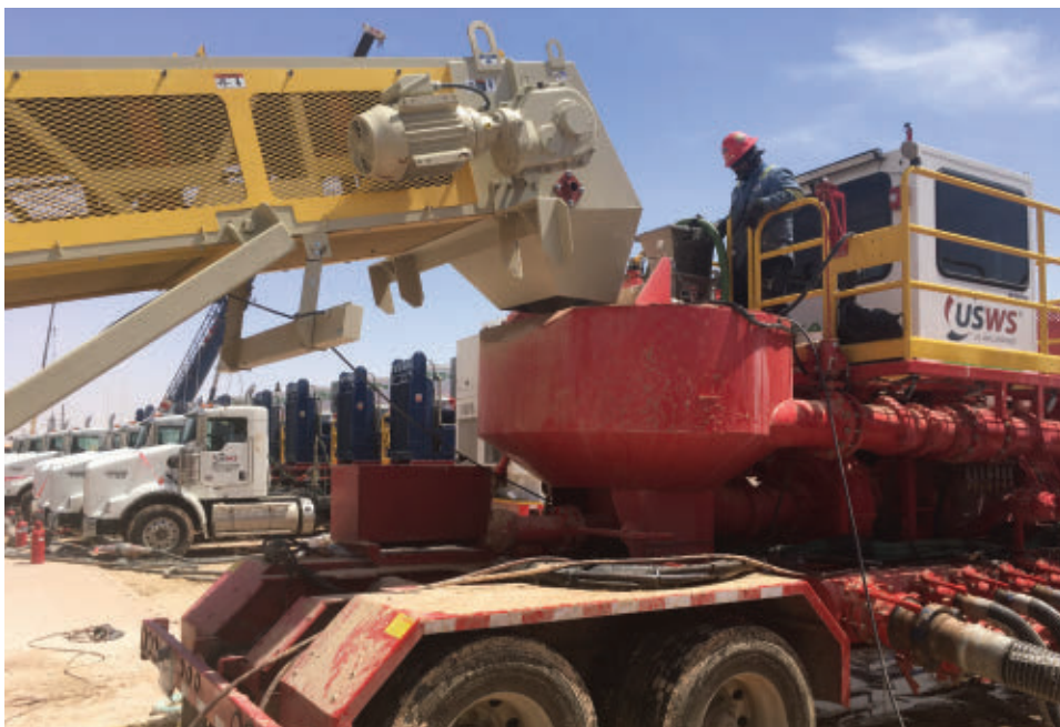
A metering conveyor replaces the auguring system on traditional blenders by using a hopper and conveyance system (Fig. 6).
